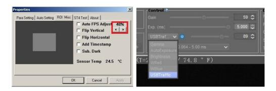
Firstly make sure the value of "Auto FPS Adjust" value is correct, this is called "USBTraffic" under Firecapture. 86% corresponds to 30fps, this value of different computers differs slightly, you can try to turn up slowly by yourself. Fluent images and no broken frame indicate that your computer have enough bandwidth for current FPS. Most computers can run steadily at 30fps, some computers can reach to 34-35fps.
