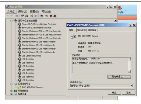
This problem probably happens when connecting camera with USB3.0 on some AMD PC or laptop. It can be solved by upgrading camera's firmware, but the speed may be slower on most computers.
