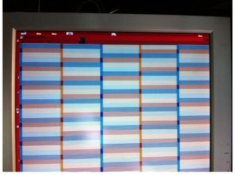
This is an incompatible problem between ASI cameras and some very old computers. It can be solved by upgrading camera's firmware, but the new firmware's speed may be slower on most computers.
